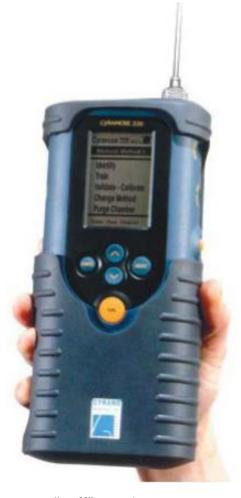
database for easy access and reporting. Rapid qualitative measurements or "sniff" tests lasting 5 to 15 seconds for discrimination and identification can be extended to quantitative headspace analyses using suitable standards for calibration.
